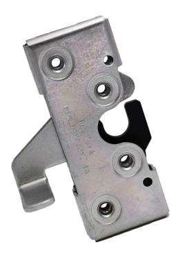
This single rotor latch is a sub-platform to the TriMark proven 050-0400 series latch and is designed for medium to heavy-duty applications for on or off-highway compartments and access panels. It features an internal trip mechanism for applications where it is desirable to have the release mechanism in-line with the latch and a two position latch.
